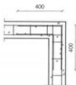
DETAIL HOEKVERBINDING RINGBALK
